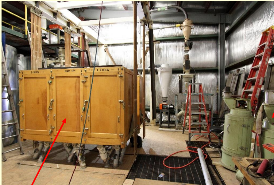
Sifter – separates flour as released from the kernel
